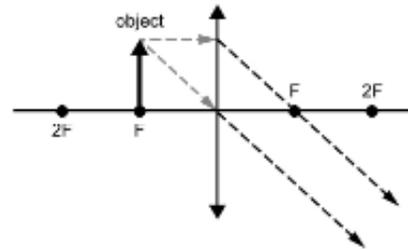
The image can't be formed because the rays entering the eye are parallel to each other. (It is also correct to say the image is virtual, an infinite size, the right way up and an infinite distance away)
