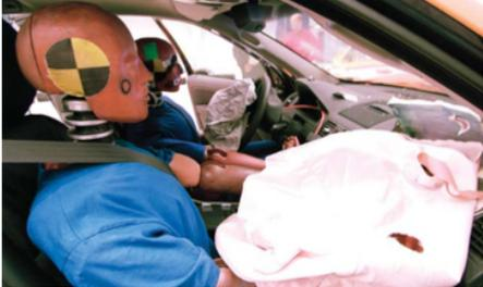
An air bag reduces the risk of damage to the head and neck.
