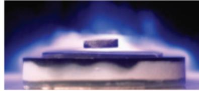
**Superconductors can be levitated with magnetic forces. This principle is used in Maglev trains.** The development of scientific ideas and discoveries has enabled us to advance new technologies, although these do
